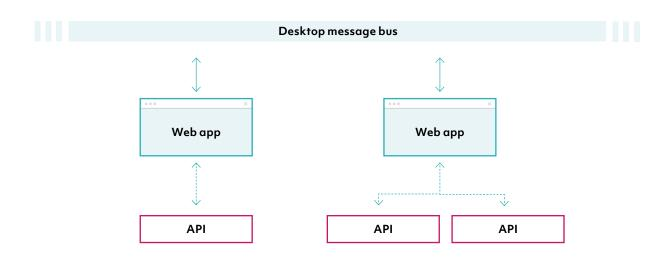
When splitting an application into a cluster of smaller applications, there is a need to support inter-app communication to allow data and events to move seamlessly from one application to another in support of user workflows. A **desktop message bus** provides this connectivity, allowing communication between applications (both bespoke and third party) entirely on the client.
