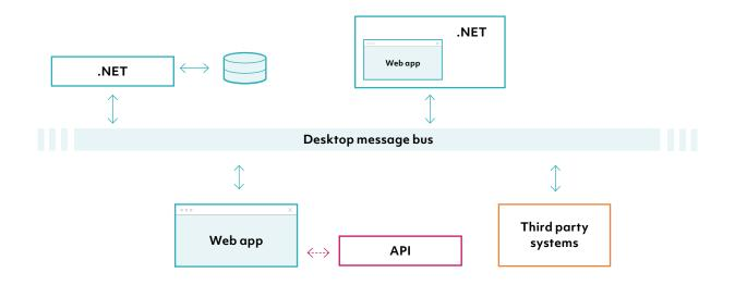
Through the use of **legacy adapters**, it is possible to exchange data between legacy applications and those running within desktop containers via the **desktop message bus**. Furthermore, various vendors provide adapters for applications that are part of the standard desktop suite, including Excel and Outlook, or finance-specific applications such as Bloomberg and FactSet.
